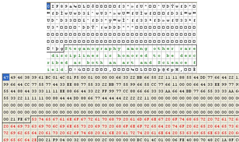
Fig. 9. Text insertion into EXIF header: (top) the inserted text string highlighted in a box and (bottom) its corresponding hexadecimal chunk.
