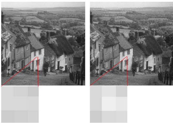
Fig. 17. Embedding at the DCT level is a very successful and powerful tool—but if coefficients are not carefully selected some artefacts will be noticeable.
