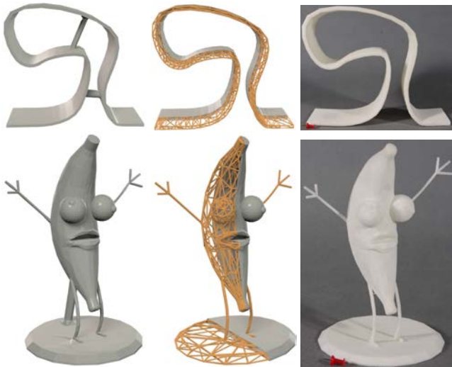
Figure 10: Left: results produced by the method of [Stava et al. 2012] by adding external struts; Middle: the skin-frame produced by our algorithm (with half-naked rendering); Right: printed objects of our results using P-1 printers.
