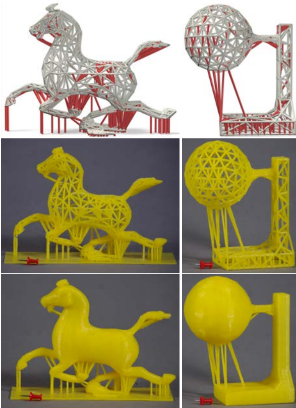
Figure 9: Printed objects using extrusion-type printers (P-2) produced by Algorithm 2. The first row shows the rendered images of the frame structures. The extra supporting struts are shown in red. With the extra struts, both the frame (the second row) and the skin-frame (the third row) can be correctly printed using P-2. The final printed models with the external supporting struts removed can be seen in the accompanying video.
