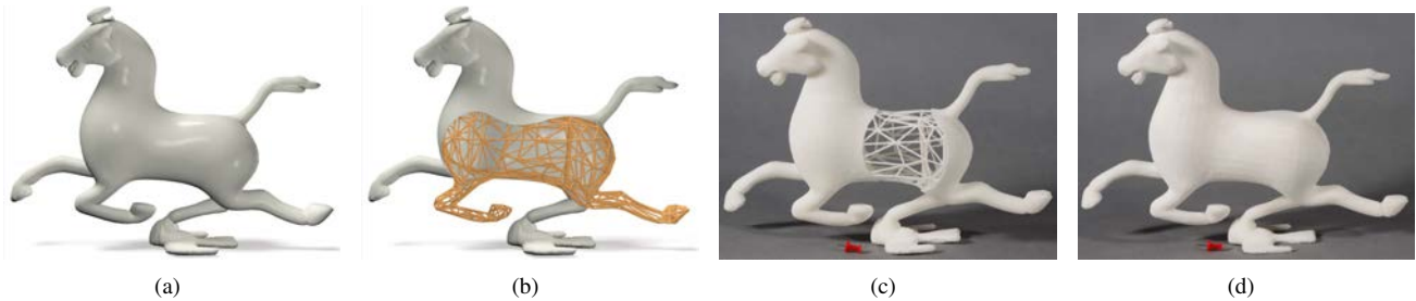
Figure 1: Given an input Horse model (a), our method generates a skin-frame structure (b), which is approximate to the model, to minimize the cost of material used in printing it. The frame structure is designed to meet various constraints by an optimization scheme. In (b) we remove the front part of the skin in order to show the internal structure of frame. (c) is the photo of an printed model by removing part of its skin to see the internal struts. (d) is the photo of the printed model generated by our method. A small red drawing pin is put under the object as a size reference in (c) and (d) respectively. The material usage in (d) is only 15.0% of that of a solid object.
