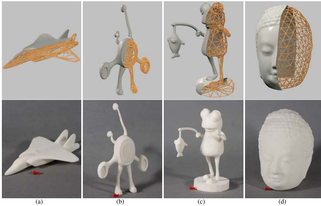
Figure 8: Printed objects using powder-type printers (P-1) produced by our algorithm. From left to right: Fighter, TV-Alien, Fishing-Frog, and Buddha-Head. The upper row shows the rendering results with half skin and half frame. The lower row shows photos of printed objects. The largest edge length of bounding box of each object is 200mm. A small red drawing pin is put beside each object as a size reference.
