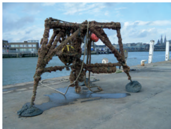
Figure 29. A tripod used for the deployment of oceanographic measuring instruments heavily fouled by hydroids (genus Tubularia ) after two months in the sea off the harbour at Zeebrugge (Belgium) in spring 2010
