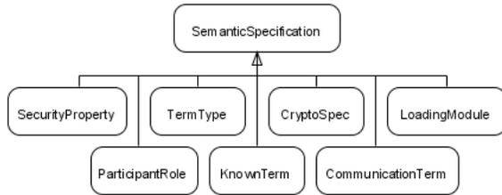
Fig. 1. Core ontology of SEM-S
