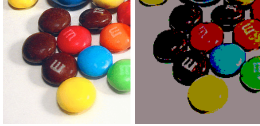
Figure 3: An illustration of the segmentation step for compressing the color space to achieve a sparse intensity representation. Left: the original image. Right: the segmentation result.
