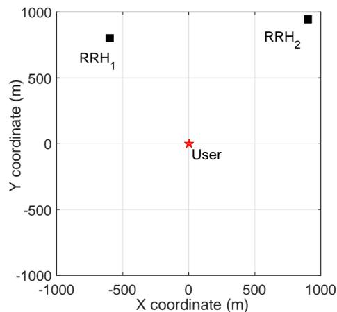
Fig. 5. Random network topology with two RRHs. The user is located at the center of the C-RAN. The coordinates of RRH 1 and RRH 2 are given by  $[-600, 800]$  and  $[900, 946]$ , respectively. The CPNRs are  $\bar{\alpha}_1 = 3.89$  and  $\bar{\alpha}_2 = 1.43$ .
