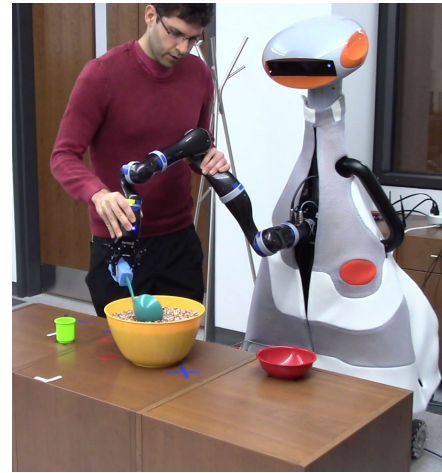
Figure 1: User teaching the robot by kinesthetic interaction
