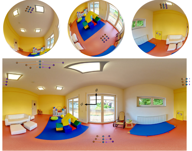
Figure 7. EquiConvs on spherical images. We show three kernel positions to highlight the differences between the offsets. As we approach to the poles (larger \theta angles) the deformation of the kernel on the equirectangular image is bigger, in order to reproduce a regular kernel on the sphere surface. Additionally, with EquiConvs, we do not use padding when the kernel is on the border of the image since offsets take the points to their correct position on the other side of the 360^\circ image.
