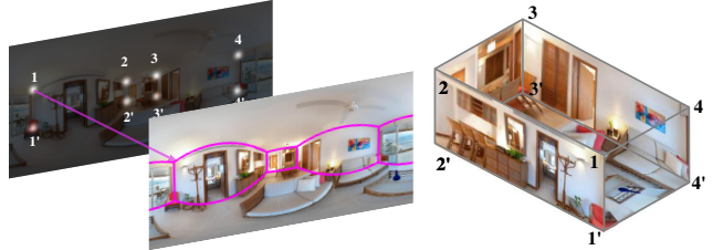
Figure 3. Layout from corner predictions. From the corner probability map, the coordinates with maximum values are directly selected to generate the layout.
