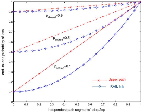
Figure 6: *The effect of shared loss.* Consider two paths with shared loss rate  $p_{shared}$  and independent loss each  $p_1 = p_2 = p$ . Here we plot the end-to-end  $p_{RAIL}$  and  $p_{single}$  vs.  $p$ , for various values of  $p_{shared}$ .
