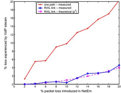
(a) Packet loss measured on each path.
