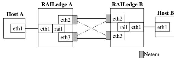
Figure 5: Experimental setup for RAIL
