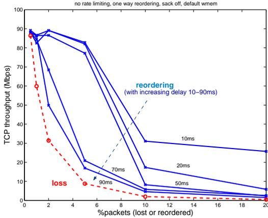
Figure 20: Testbed experiments comparing the effect of loss vs. reordering on the throughput of a single TCP flow.
