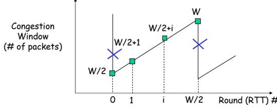
Figure 17: The simple steady-state model for TCP [29].
