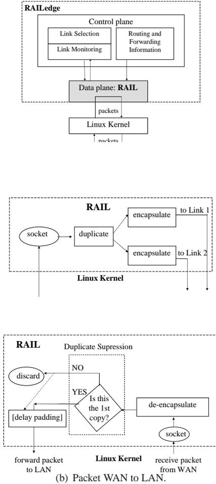
Figure 3: RAIL functions upon reception of a packet.
