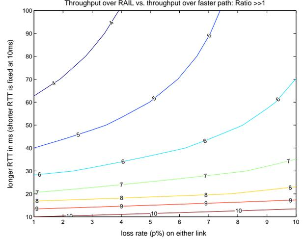
Figure 18: Consider two paths with the same  $p$  and different  $RTT_1 < RTT_2$ , for the full range of  $p$ 's and  $RTT$ 's. The figure shows the ratio of TCP throughput over RAIL vs. tcp over the fast link. RAIL performs roughly 10 times better for the range of practical interest.
