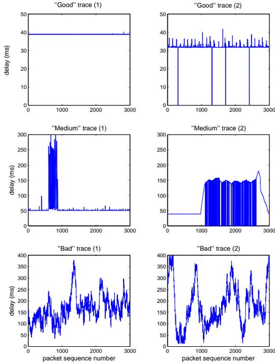
Figure 11: Six representative packet traces, collected over wide-area paths of Internet backbones [28]. We plot one-way delay vs. packet sequence number; when a packet is lost we give it a 0 value.
