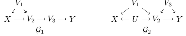
Figure 4: Two DAGs: in \mathcal{G}_1 all variables are observed, in \mathcal{G}_2 variable U is unobserved. We assume \mathbf{I} = \emptyset . For \mathbf{X} = \{X\} and \mathbf{Y} = \{Y\} FINDMINSEPINDAG computes in \mathcal{G}_1 separator \{V_2\} , resp. in \mathcal{G}_2 separator \{V_2, V_3\} .
