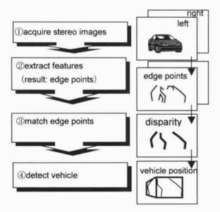
Figure 2. Vehicle position estimation using stereoscopic distance measurement
