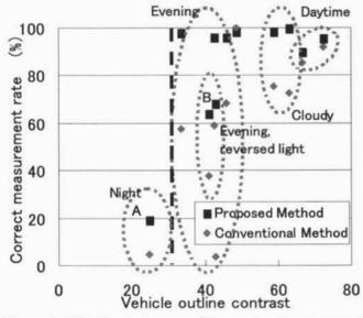
Figure 7. Relation between outline contrast and correct measurement rate
