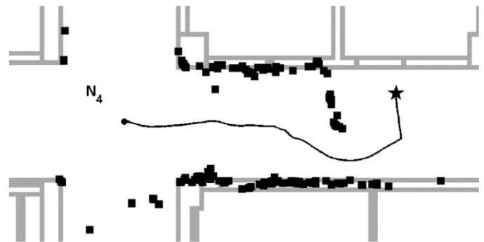
Fig. 13. As in Fig. 12, this figure shows the robot navigating to the goal on the final edge. However, the path is partially obstructed by an obstacle that was not present when the map was created. The goal meet point is shown by a dark circle and the goal location by a star. Filtered sonar points are represented by dark squares.
