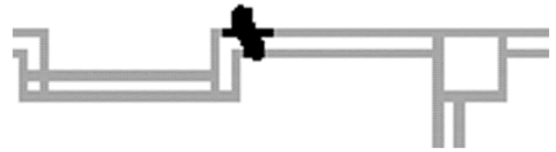
Fig. 8. Landmark location indicated in Fig. 7 is shown in greater detail, demonstrating the inconsistency between the edge map and the floor plan. The corner of the doorway should lie at the location of the landmark.
