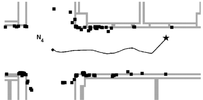
Fig. 12. Sonar map as the robot traveled along the final edge of Fig. 9 to the goal is shown. The goal meet point is shown by a dark circle and the goal location by a star. Filtered sonar points are represented by dark squares.
