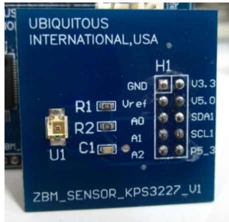
FIGURE 7. The KPS-3227 Illuminance Sensor
