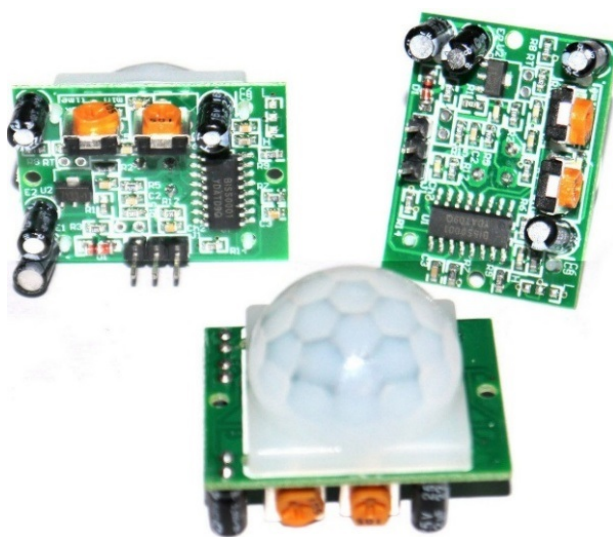
FIGURE 4. HC-SR501 Human Detection Infrared Ray Sensor
