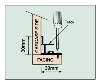
The Kethy Tambour door has many comercial applications providing an elegant finish to any cabinet. The fitting of locks will provide added security if desired.
