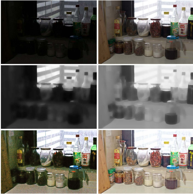
Figure 3: Left column: Lower light input and its decomposed illumination and (degraded) reflectance maps. Right column: Brighter input and its corresponding maps. Three rows respectively correspond to inputs, illumination maps, and reflectance maps. These are testing images.
