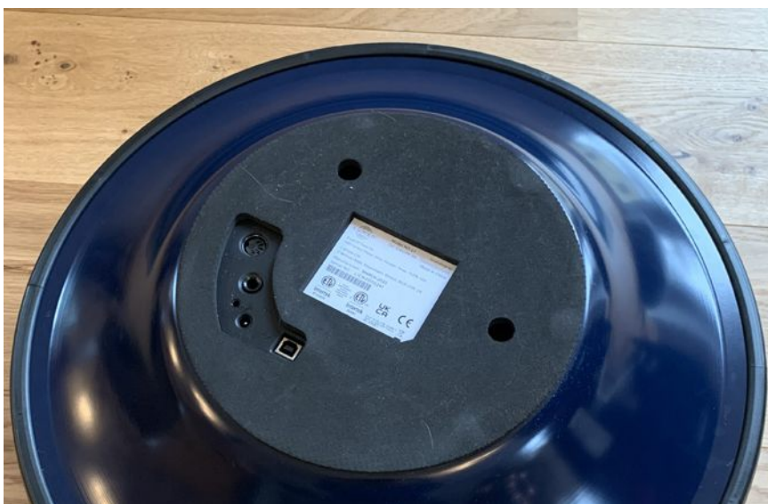
■ The rear — or under — panel includes a MIDI out port, quarter-inch audio output, a socket for the external PSU and a USB-B port for charging and interfacing with a computer.
