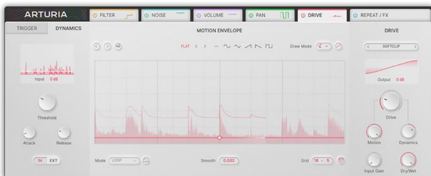
The Motion Envelope for each module can be triggered in a variety of ways including based upon the dynamics of the input signal.
