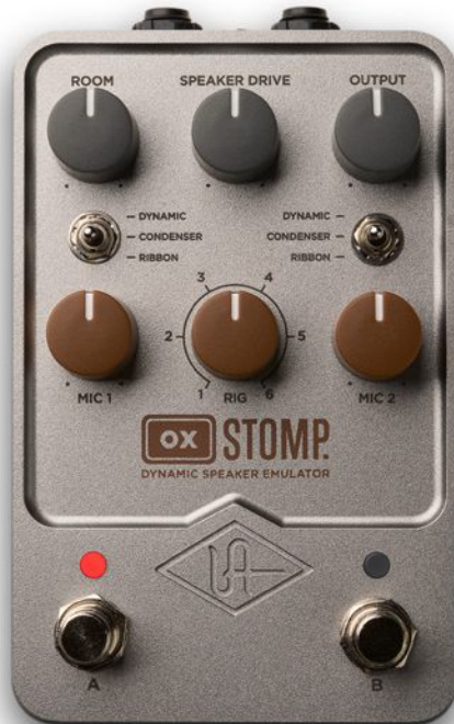
— The OX Stomp has a limited number of physical controls on board, with much deeper, detailed control and editing available via the UAFX Control app.
