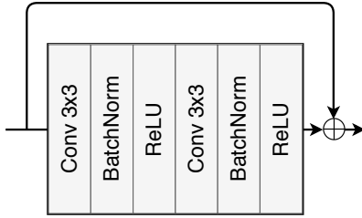
Figure 3: Architecture of a residual block
