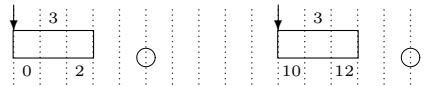
Figure 1.3: Two requests of a single task, the first one occurs at time 0, the second one at time 10.
