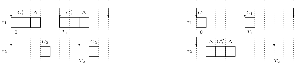
Figure 2.5: Schedule of task set \{\tau_1, \tau_2\} , if C_1 = T_2 - T_1 + \Delta (left) and C_1 = T_2 - T_1 - \Delta (right).
