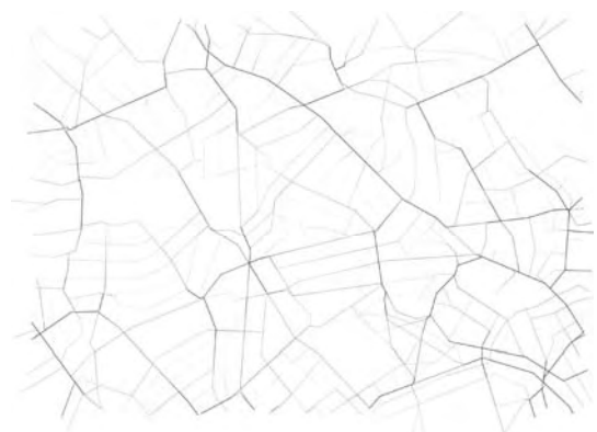
Figure 1.12b Choice analysis of part of north west London for trips up to 1.25km
