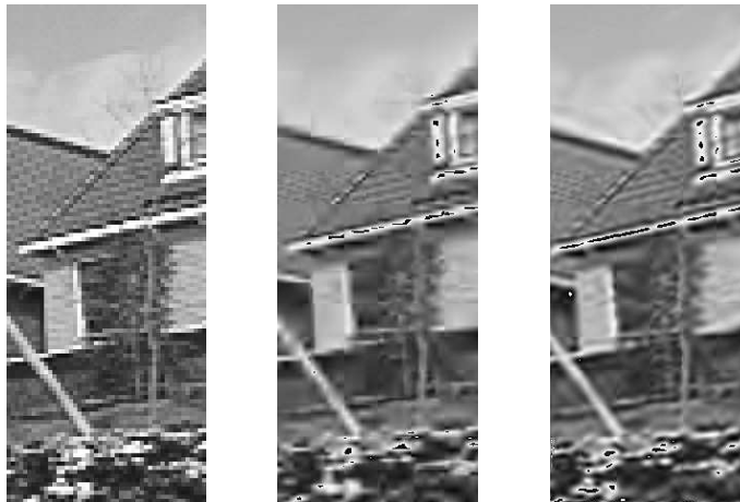
Figure 7. (a) Original frame; (b) Higher resolution version using spline interpolation; (c) Higher resolution version using GROW.
