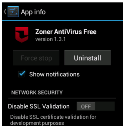
(a) Developer settings to turn off certificate validation for an app. This option is not displayed for normal users.
