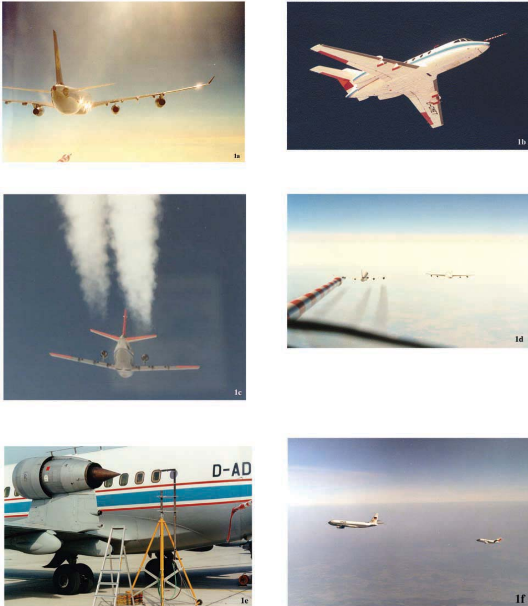
Figure 1. (a) Photo of the Airbus A340 at cruise during S7 measuring about 70 m behind the right turbofans. The nose boom of the Falcon used for turbulence measurements is visible at the lower edge of the photo; (b) the Falcon with particle measurement systems below the wing and aerosol inlet at top of the fuselage during S4; (c) the ATTAS at cruise during S2 burning low (high) fuel sulfur content on left (right) engine; (d) the A340 and the B707, wing by wing, one with, the other without contrails during S7; (e) sample inlet behind the ATTAS engines at ground during S3; (f) Falcon measuring in the B707 plume 70 m behind the engines during S7.
