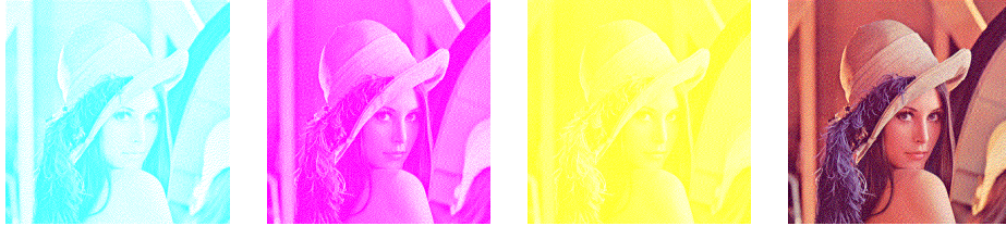
Fig. 9. Dithered C , M and Y Components and their Superimposition
