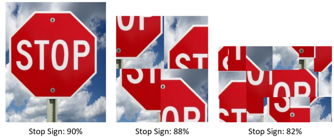
Fig. 2: An example showing how object classifiers are only concerned with matching geometry. In this case, Google Cloud’s Vision API is used: https://cloud.google.com/vision/ .
