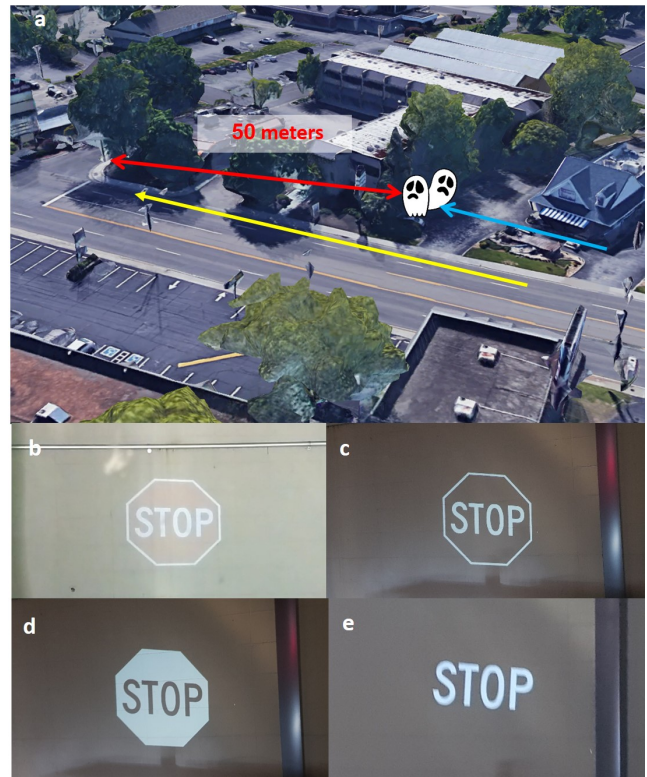
Fig. 23: Fooling the stop sign recognition system: Each of the four phantoms (b-e), projected for just 125 ms, were recognized by Tesla's stop sign recognition system. The phantoms were projected on a white wall located 50 meters from a nearby intersection that contained a real stop sign.
