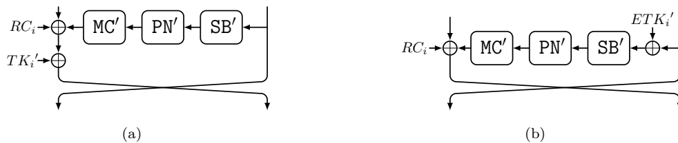
Figure 3: The round function for weak tweak-key CRAFT.
