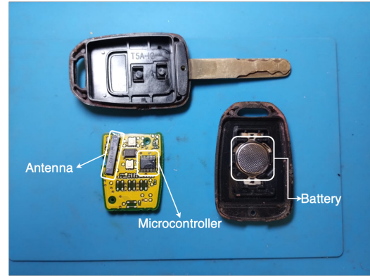
Figure 1. The Components of the disassembled Honda key, the main components are the Coin Cell Battery, the Micro-Controller and the Antenna.
