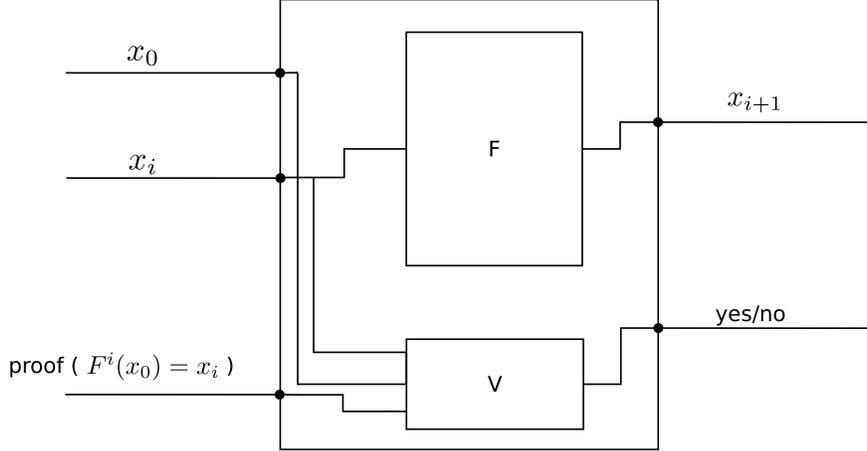
Figure 3: Illustration of recursion-based IVC.  $F$  is the circuit computing the loop iteration,  $V$  is the verifier circuit verifying a proof for  $F'$ , the illustrated circuit itself. The public input is  $x_0$  along with the public outputs  $x_{i+1}$  and the verifier output, the other two inputs are prover inputs.
