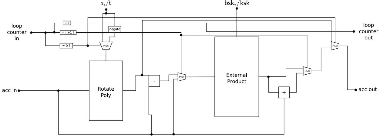
Figure 4: IVC Circuit for TFHE’s PBS. This corresponds to the subcircuit F from Figure 3. We omit the hash chains over the bootstrapping key and ciphertext  $(\mathbf{a}, b)$ . The mod switch is not depicted since we consider it integrated into the polynomial rotation as described in Section 4.1.
