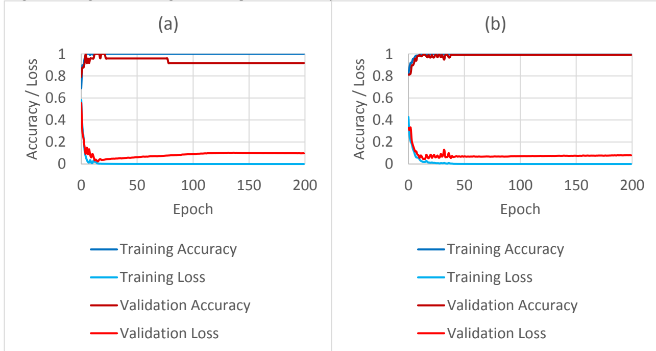
Figure 6 CNN-LSTM network performance (accuracy and loss function for both training and validation) when using 2s long inputs (a) and 0.5s long inputs (b)
