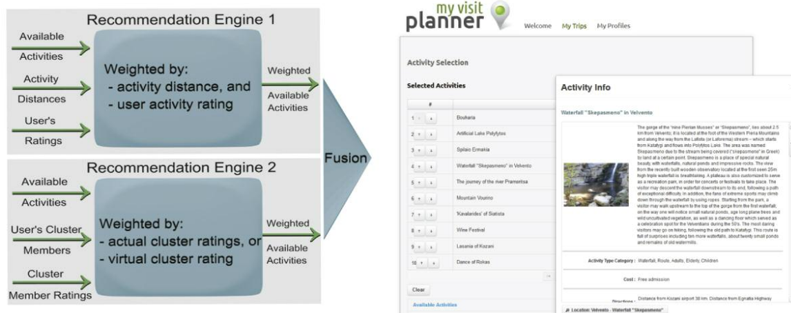
Figure 2: Recommendation engine principle and interface for reviewing recommendations.
