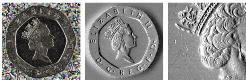
Figure 3: Coin texture (left) and fine surface detail contributed by photometric stereo (middle and right) as recorded by our approach.
