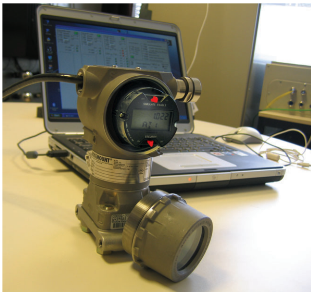
Figure 1: The new pressure controller system in the testbed environment.
