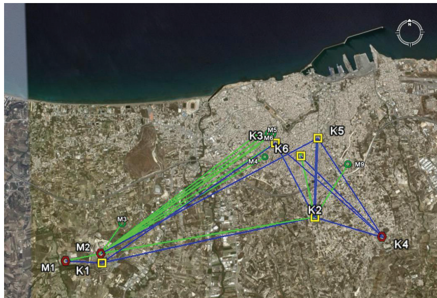
Figure 1: The experimental metropolitan wireless multi-radio mesh testbed in Heraklion, Crete. The mesh testbed contains IEEE 802.11a links with lengths ranging from 1.6 to 5 km. Nodes K1-6 are core mesh nodes, while nodes Mx are used for management and monitoring.
