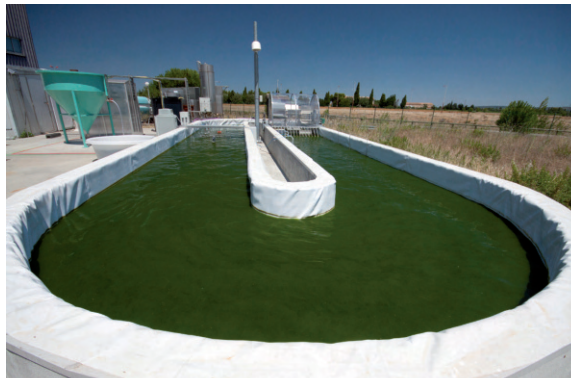
Figure 1: A typical raceway for cultivating microalgae. Notice the paddlewheel which mixes the culture suspension. Photo: INRA
