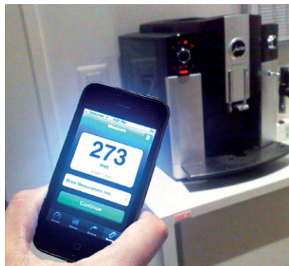
Figure 2: Measuring the standby power of a specific household appliance
