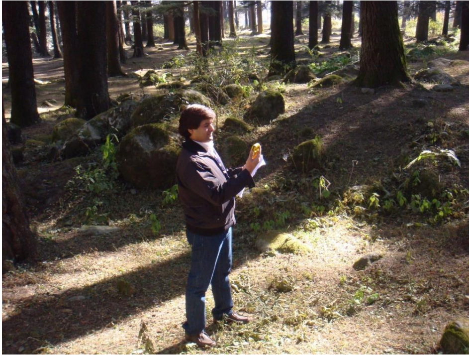
Figure 11: Figure showing Dr. Shashi Kumar using a laser dendrometer RD1000 to obtain the tree heights within a plot of 0.1 hectare. Image was taken on 27 November 2012.
