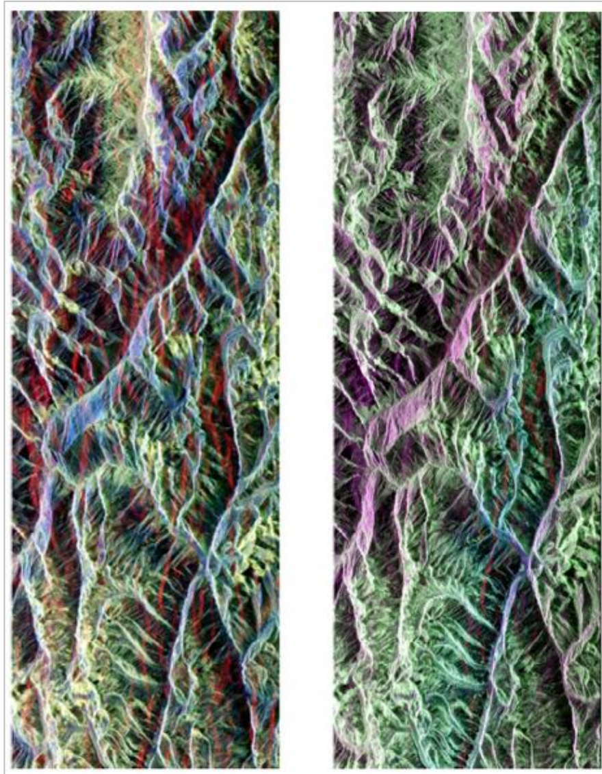
Figure 17: Pauli RGB images of ALOS-2 data. Left side: S1 scattering matrix, right side: S2 scattering matrix. Note that, image is inverted vertically because terrain correction was not performed in this step. Here, red: double bounce scattering component, blue: surface scattering component, green: volumetric scattering component, and white: presence of all the scattering components equally.
