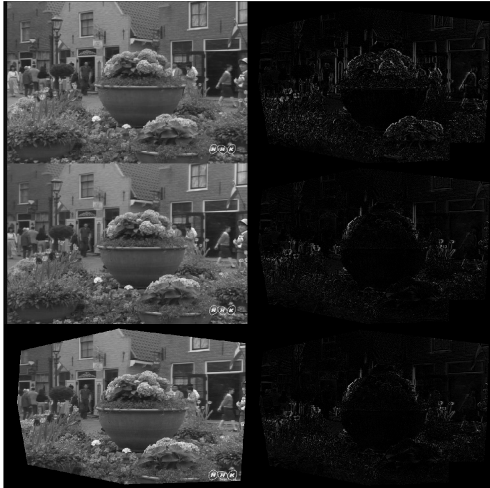
Figure 4.17: Flowerpot. Left column, top to bottom: Reference, target and predicted frames. Right column, top to bottom: Initial error, error before nonlinear stage, error after nonlinear stage.
