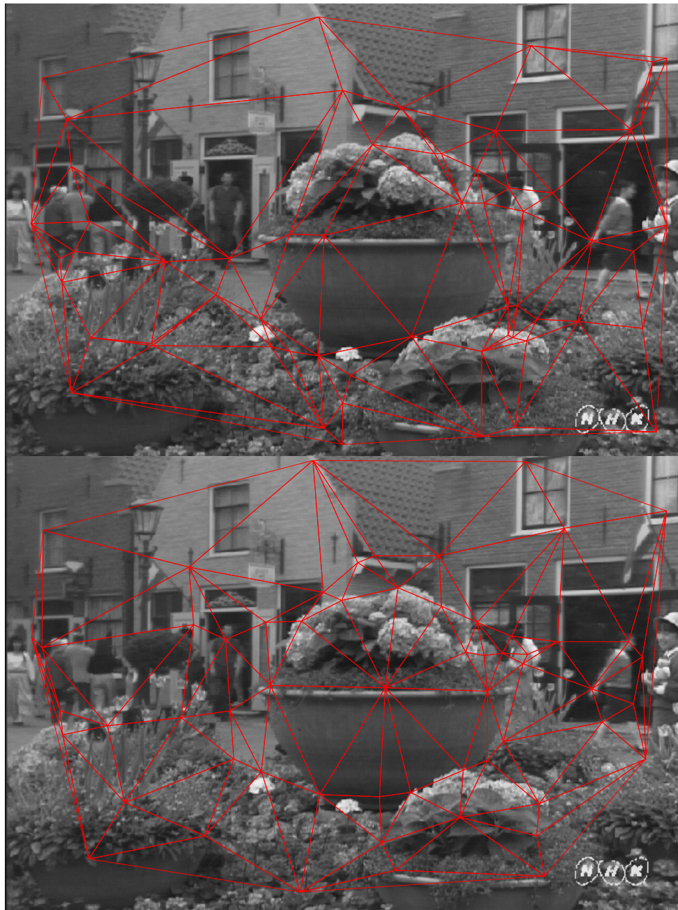
Figure 4.26: Manual vs. automatic mesh determination in Flowerpot . Top: Planes recovered by the algorithm. Bottom: Planes recovered by manual selection of the points.
