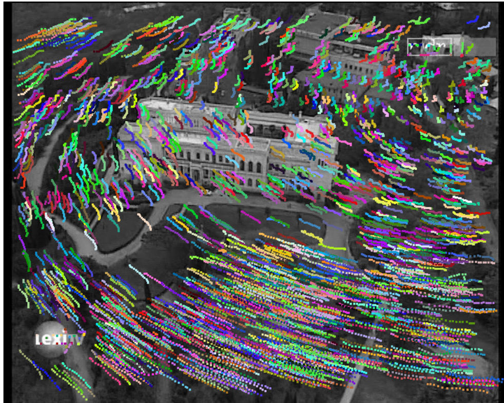
Figure 2.7: Results for OF tracking. Each color indicates a feature trajectory, and each square, a point on the trajectory of that color.
