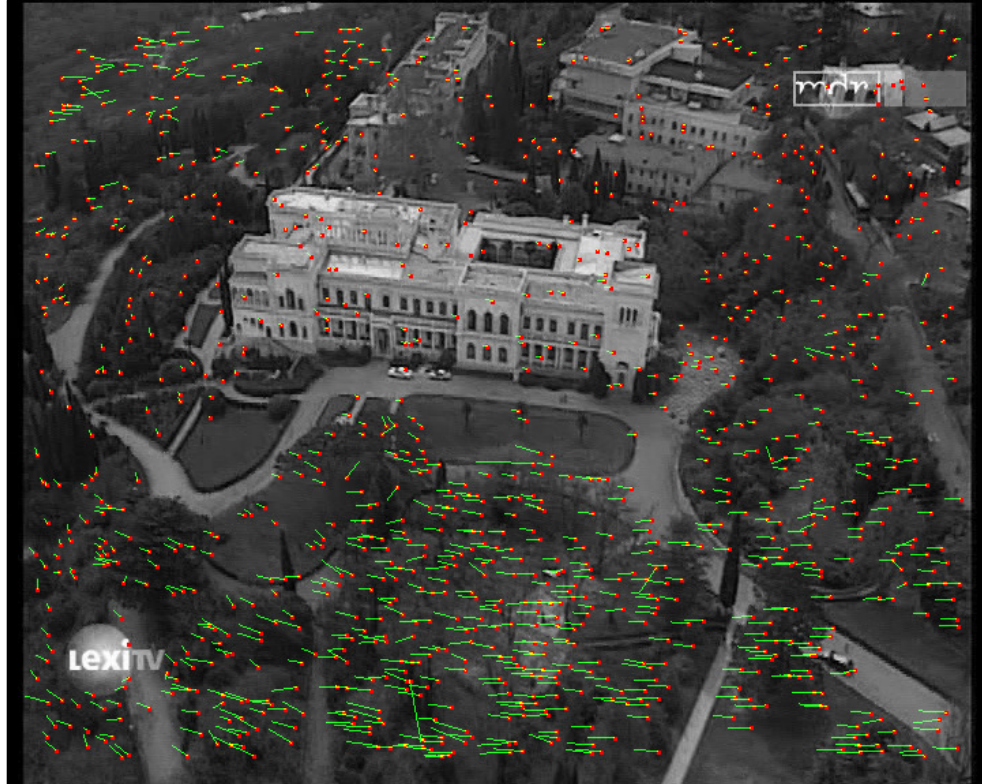
Figure 2.5: Feature displacements estimated by KLT. Red squares indicate the features, and green lines, the displacements. Displacement magnitudes are scaled by 4 to enhance visibility.
