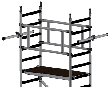
14) Fit 2 side props every 2m, one either end of the tower. If you cannot fit side props, stabilizers shall be fitted to all 4 corners of the tower. They shall be fitted to create the largest footprint possible.
