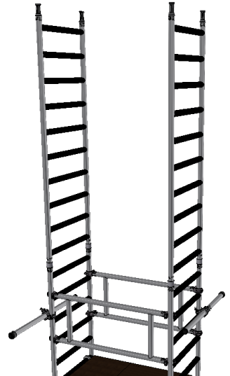
15) Fit a additional frames and engage the interlock clips.
