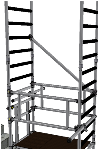
11) Fit a diagonal brace from the top rung of the frame below.
