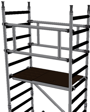
13) Sitting through the platform, fit 2 guardrail frames, one either side or 4 Horizontal braces 2 either side with hooks facing out.
