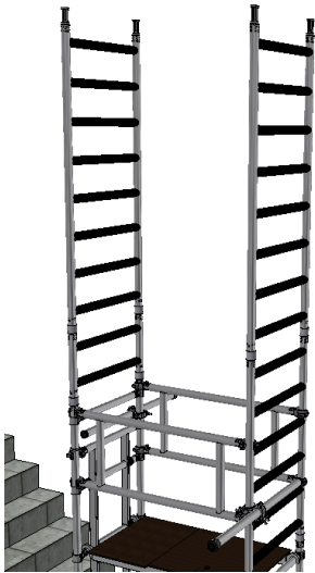
10) Fit a additional frames and engage the interlock clips.
