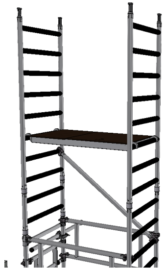
12) Fit a trap platform to the 6th rung down from the top when installing on a FKS4/8.
