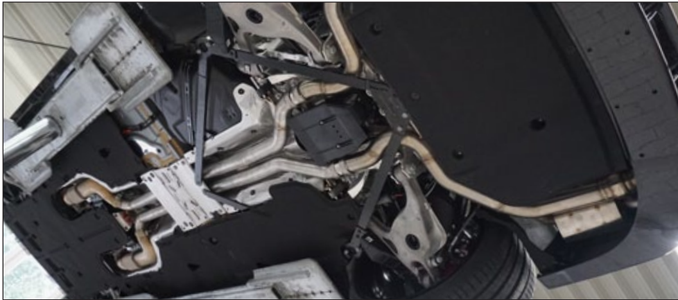
Sport Exhaust System with manuel switch for MANSORY rear bumper FS2 255 460 left & right Sport Muffler with throttle control
