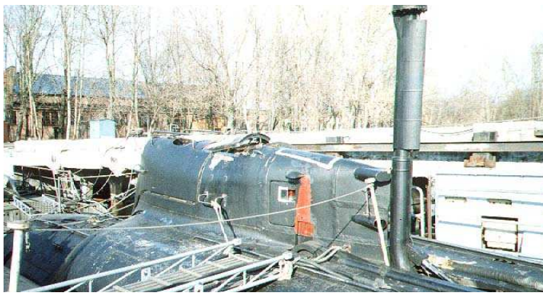
Pyranja (snorkel reses hydrauliskt) http://submarine.id.ru/galery/t317.shtml
