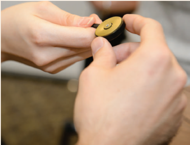
THIS TACTOR, SIMILAR TO THE TECHNOLOGY THAT MAKES A CELL PHONE BUZZ, IS DESIGNED SO THAT RIGGS CAN MANIPULATE PARAMETERS LIKE AMPLITUDE, FREQUENCY, AND PULSE PATTERN.
