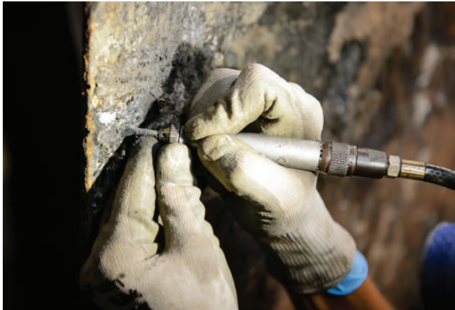
A thick, hardened coat of sand, sediment, and shell, the concretion on the sub is being carefully chiseled away.
