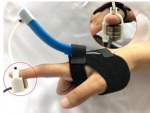
Fig. 13. The setup to measure the force exerted by the rigid rod on the user's fingertip, while the zoomed view shows the force sensor
