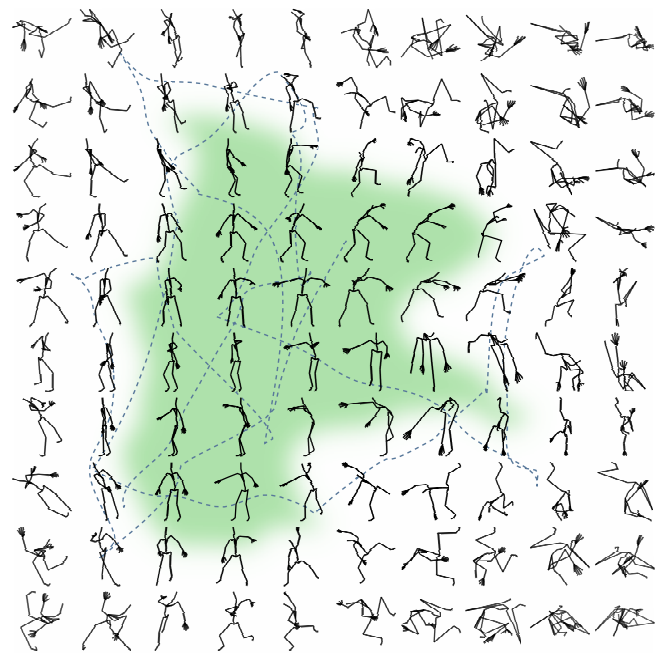
Figure 1: An example of a 2D pose map and a generated movement path. The low dimensionality enables a graspable illustration; in the actual experiments, a 7D map was used. The green area represents the region of observed poses, while the surrounding areas contain poses without any direct equivalents in the training data. The blue dotted line represents an example of an automatically generated trajectory with a high novelty parameter. As seen in the illustration, the novelty constraint causes the path to stretch beyond observed territories. (The visualization uses a grid of poses but the actual pose map is an unbounded continuous space.)
