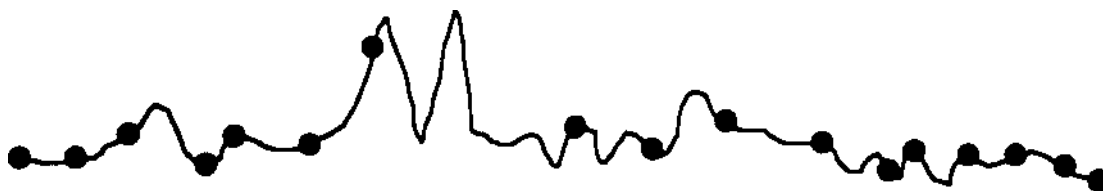
Figure 3: Polling. The input data are sampled whenever the system finishes processing the previous data.
