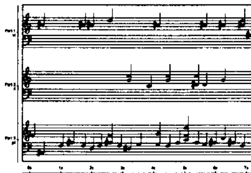
Figure 7: A part of results yielded by the implemented system. A note value recognition (e.g. quarter notes, half notes, ...) is not considered here and all the notes are displayed as quarter notes with a real-time scale.
