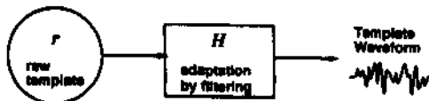
Figure 1: A sound source model that consists of a template r and an FIR filter H . Here, H modifies the waveform of the original template r to cope with variation of a sound.
