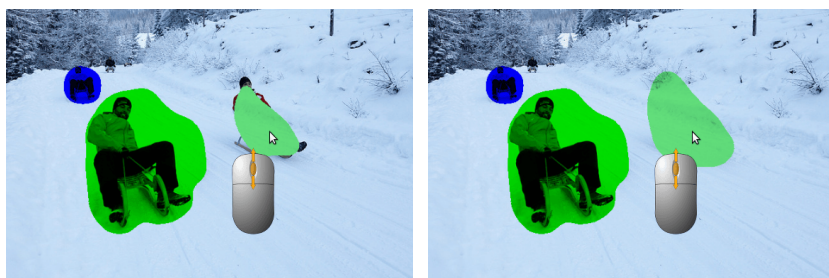
(a) Mouse wheel scroll in one direction to increase the global threshold (b) Mouse wheel scroll in one direction to decrease the global threshold
