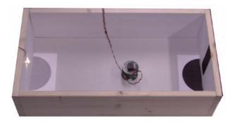
Figure 4. A mobile robot Khepera equipped with a vision module can gain fitness points by staying on the gray area under the light bulb *only* when the light is on. The light is normally off, but it can be switched on if the robot passes over the black area positioned on the other side of the arena. The robot can detect ambient light and wall color, but not the color of the floor.
