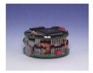
Figure 1. The miniature mobile Khepera robot has a diameter of 6 cm. It is equipped with two wheels and 8 active infrared sensors (6 on the front and 2 on the back) that can measure distance from objects or the amount of ambient light.
