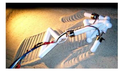
Figure 3. An evolved morphology. The control system consists of a neural network driving the central actuator in perfect anti-phase with the two synchronized lateral limbs so that while the upper two limbs push, the central body is retracted, and vice-versa. Figure courtesy of Hod Lipson and Jordan Pollack. Reprinted with permission.
