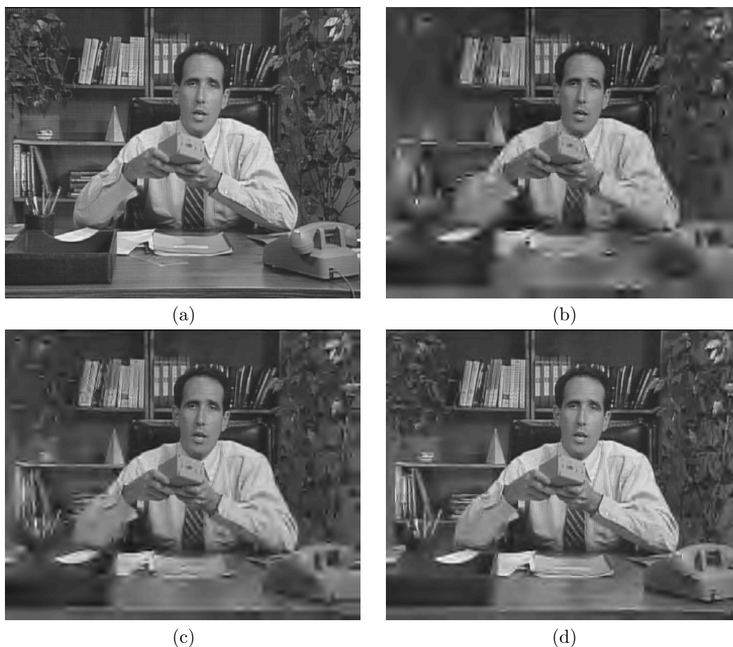
Fig. 13. Frame 32 of the “Salesman” sequence (a) compressed using FSVC at 200 Kbits/sec (b), 400 Kbits/sec (c), and 800 Kbits/sec (d), respectively.
