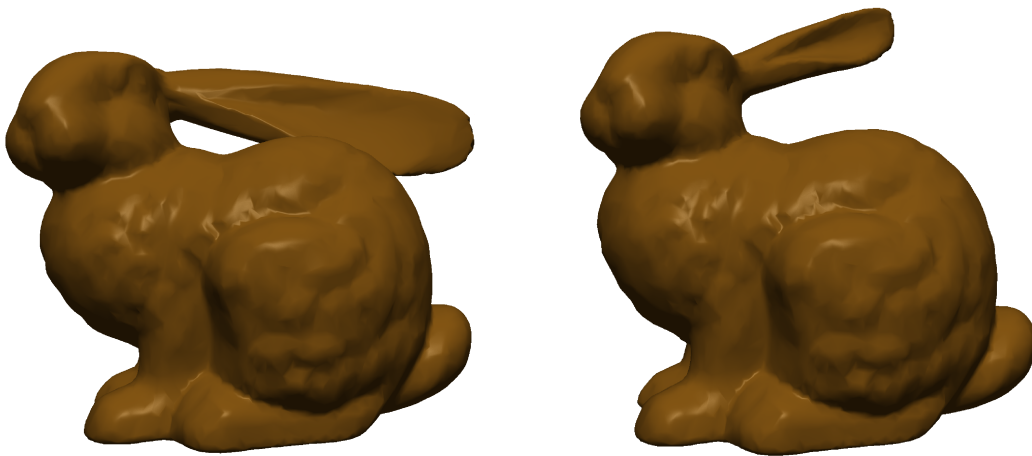
Figure 2.3: The images show the displacements due to external forces as they were simulated using the linear Cauchy strain tensor (left) and the non-linear Green strain tensor (right).
