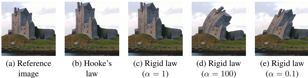
Figure 2.9: Modified material laws in 2D: Images (b) and (c) show the difference between Hooke's law and the rigid law if the castle is stretched vertically. Images (d) and (e) demonstrate the effects of reducing the amount of shearing (d) and rotation (e) while the castle is dragged to the right.
