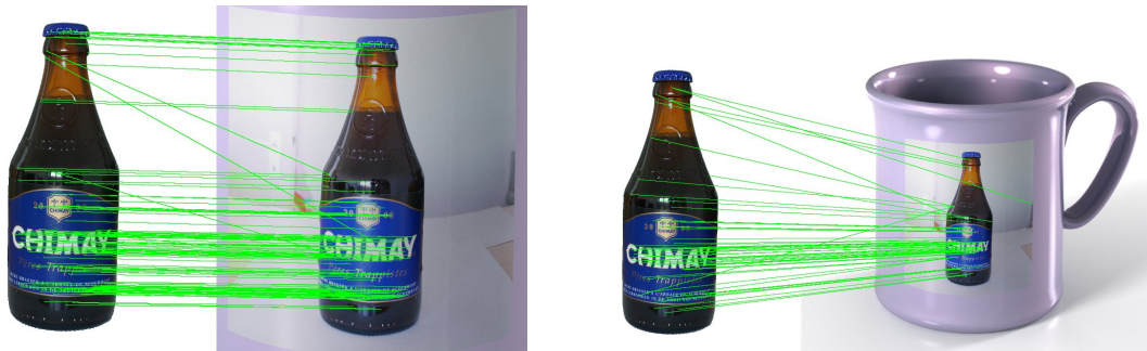
Figure 1.2 An example of a good model match using features extracted from 2D images (left), where a beer bottle template is successfully identified in an image. However, zooming out from the image, we observe that the bottle of beer is in fact another picture stitched to a completely different 3D object (in this case a mug). The semantics of the objects in this case are thus completely wrong.
