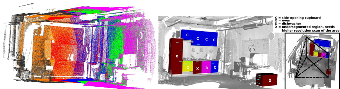
Figure 5.2 Left: The registration of the six datasets from Figure 5.1 into a consistent and complete point cloud model. Right: a segmentation example describing furniture candidates identified in the data.
