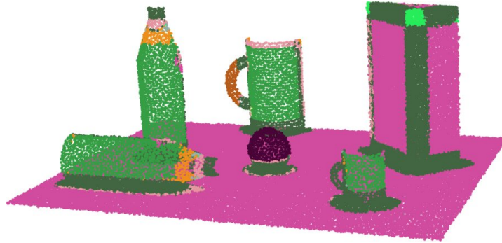
Figure 8.12 Complex noisy synthetic scene with 90.26% classification results using a sublinear SVM kernel.
