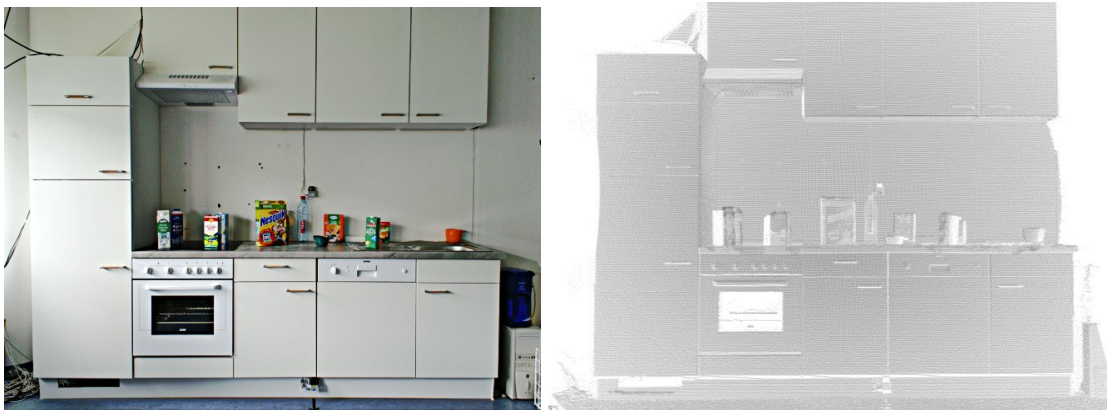
Figure 6.1 Left: a kitchen scene, right: the resultant point cloud dataset representing the kitchen.
