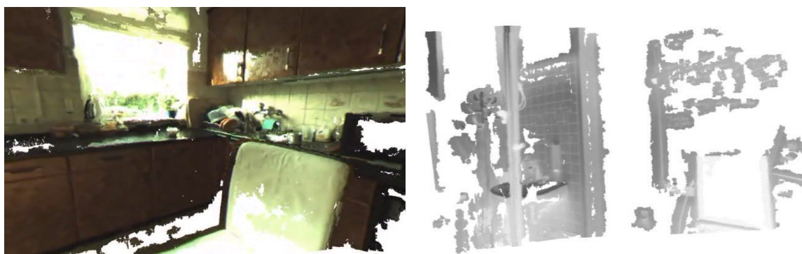
Figure 2.5 Examples of point cloud datasets acquired using a stereo camera: in a textured environment (left); in an environment that lacks texture information in certain regions (right).
