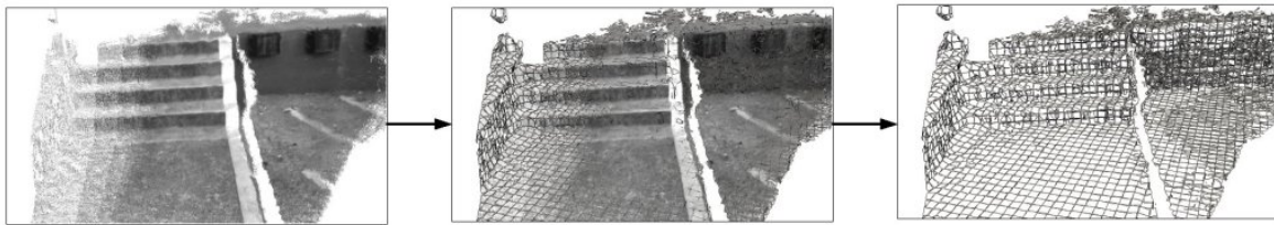
Figure 12.10 Point Cloud model simplification using polygonal fitting. From left to right: overlapping aligned point cloud views, combination point cloud data model and polygonal model, and the resulting polygonal model.
