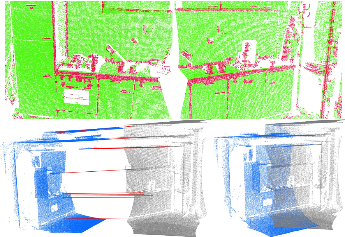
Figure 5.3 Aligning two scans of a kitchen dataset using a set of good PFH correspondences. The persistent PFH representations selected as interesting points for registration are shown at the top.
