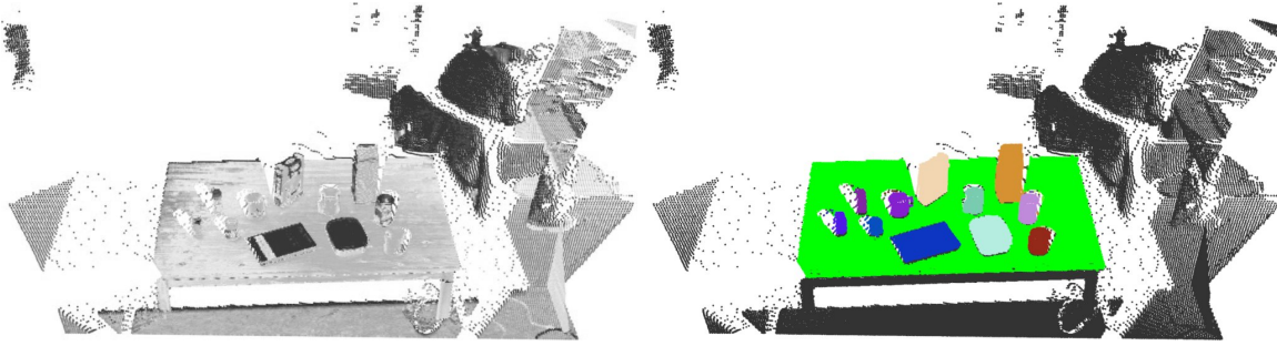
Figure 8.17 Left: raw point cloud dataset; right: the segmentation of the table (green) and the objects supported by it (random colors) from the rest of the dataset (black).
