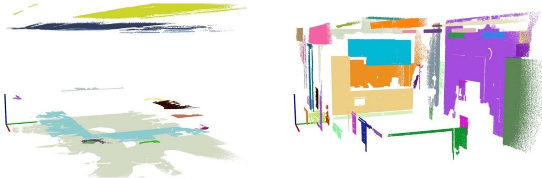
Figure 7.13 Left: all horizontal planes found in the scene; right: all vertical planes found in the scene.
