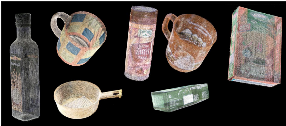
Figure 2.1 Example of very accurate point cloud datasets representing objects found in kitchen environments, acquired using structured light sensing devices.
