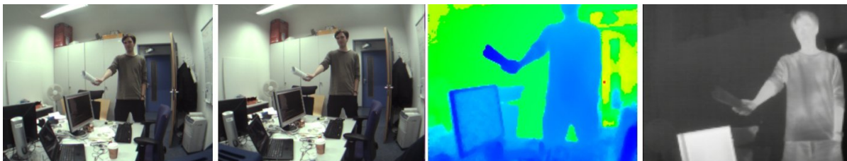
Figure 2.7 Different images taken using the composite sensor device from Figure 2.2. From left to right: stereo camera left and right images, TOF camera depth image, and finally a thermal camera image.
