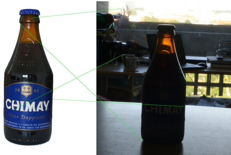
Figure 1.1 Model matching failure in underexposed 2D images. None of the features extracted from the model (left) can be successfully matched onto the object of interest (right).
