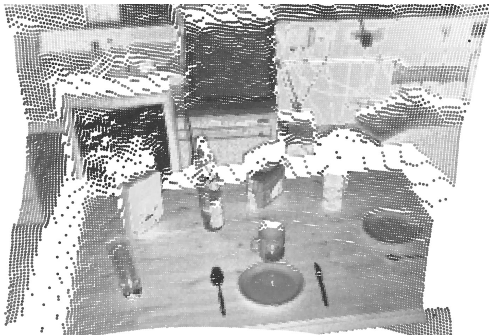
Figure 2.4 An example of a point cloud dataset acquired using a Time-of-Flight camera.
