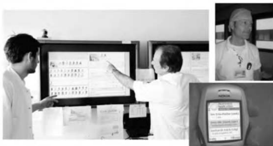
Figure 1 - The AwareMedia System running on two large displays in use at the hospital (left), The AwarePhone System displaying a list of clinicians and their location (bottom) and at the top is a clinician wearing a small tracked Bluetooth chip (top)
