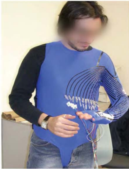
Figure 2 – Sensorized garment for motor rehabilitation. Picture of an early prototype whose CE tracks are visible.
